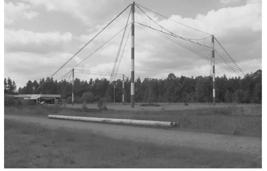
Fig. 2. Open area TEM waveguide at the WIS, Munster, Germany.
